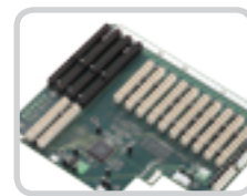
Flexible board configuration between industrial motherboard (IPPC-7157A) or passive backplane (IPPC-7158B)
